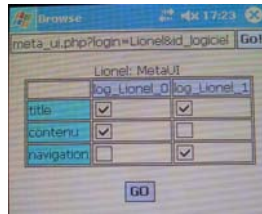
Fig. 4. Additional UIs for the end-user: the check boxes represent the mappings between the UI structure (the rows: title, content, navigation) and the connected platforms (the columns).
